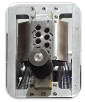
The ultrasonic probes are positioned within the probe holders at specific intervals to ensure uniform and complete coverage of the billet surface.
