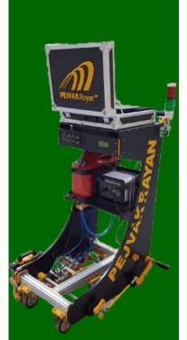
With this device, the user can inspect plates at an adjustable scanning speed of up to 30 meters per minute, which significantly increases inspection speed and efficiency compared to manual methods.
